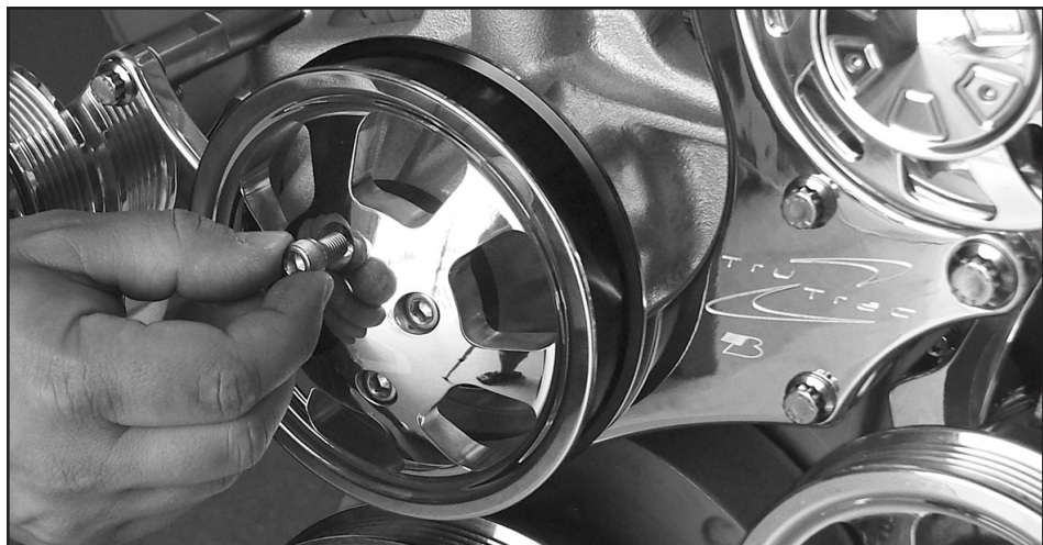
Figure 9: Install Water Pump Pulley onto Pump
