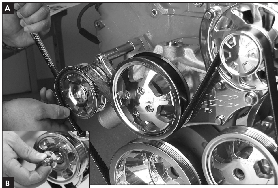
Figure 11: Install Serpentine Belt & Tensioner Pulley
