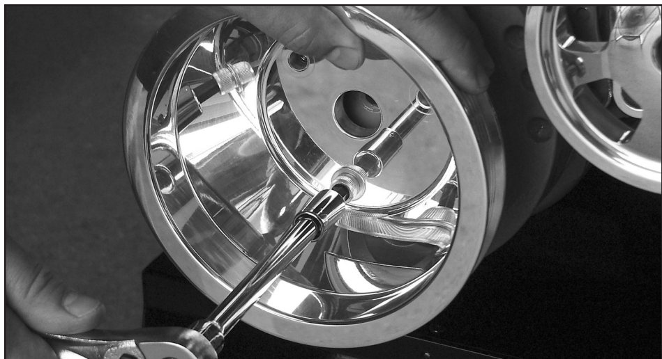
Figure 10: Install Crankshaft Pulley
