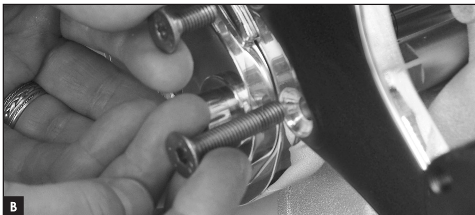
Figure 7: Attaching Bridge Bracket
