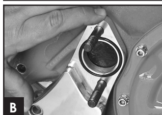
Figure 2: Install Tensioner Support & Alternator Bracket
